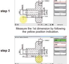
Measure the 2nd dimension by following the yellow position indication. The 1st data will be shown in red or green according its tolerance.
