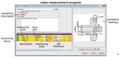
Make measurement program for each one inspection computer. Maximum 200 dimensions can be measured by one inspection computer.
